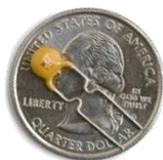
Figura 1.98 – Um PTC de 500 mA. Fonte: [www.sparkfun.com/tutorials/57](http://www.sparkfun.com/tutorials/57).
